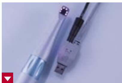
The voltage supply of the VistaProof is provided by separate power supply directly at the USB connector - conforms to MPG.
