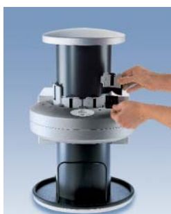
1. Insert the image plate into the foil cassette
